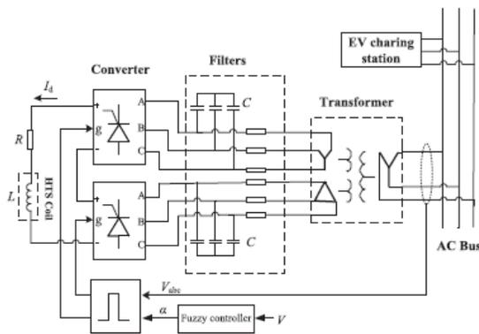
**Fig.3.1. Proposed system Block diagram.**
