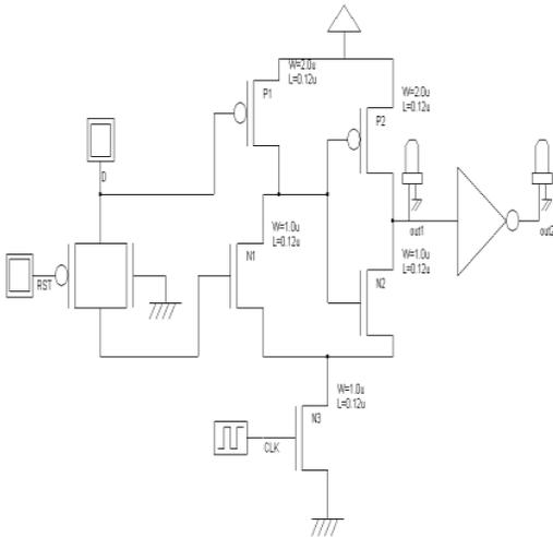
Fig.2.proposed low power clocked pass transistor flip-flop
