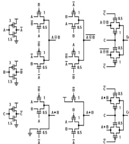
**Fig.2. Full-adder designed with the Energy Efficient structure using a DPL logic style.**
