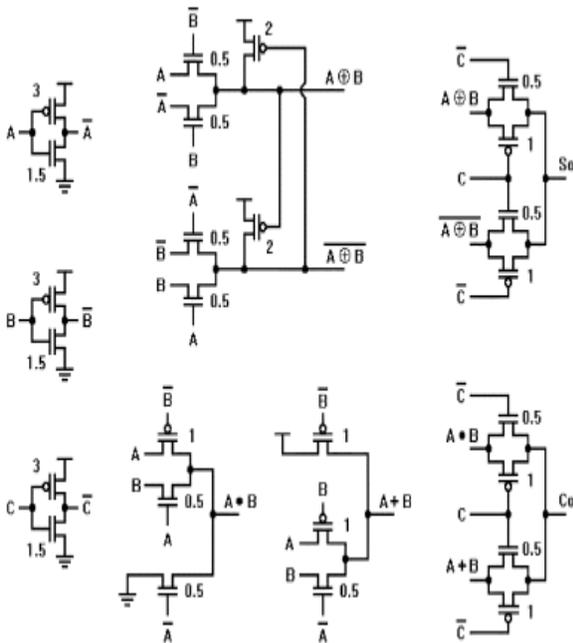
Fig.3. Full-adder designed with the Energy Efficient structure using a SR-CPL logic style.
