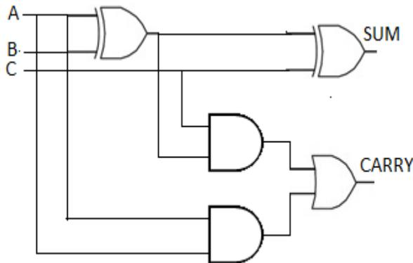
**Fig.1. Logic diagram of a full adder.**
