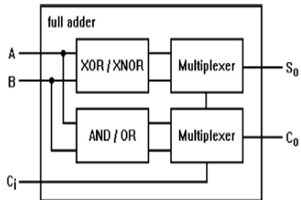
**Fig.2. Alternative Logic scheme for energy efficient full adder.**
