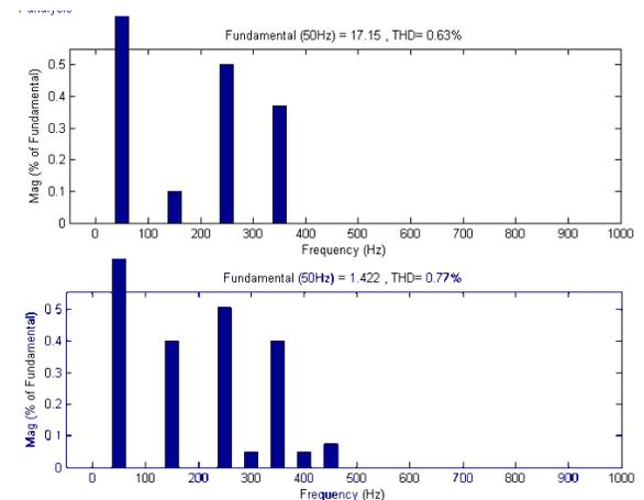
Fig. 7. Stand-alone mode with a resistive load. (a) (Upper)  $u_A$  and its reference  $u_{ref}$  and (lower) current  $i_A$ . (b) (Upper) Voltage THD and (lower) current THD.
