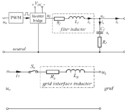
Fig. 3. Control plant Pi for the outer current controller.
