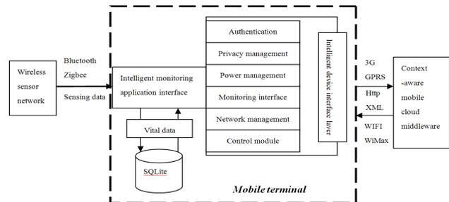
Figure 2: Sensor and mobile sensing data flow diagram
