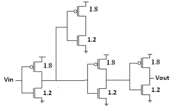
Figure 4. Equivalent circuit for Design2.
