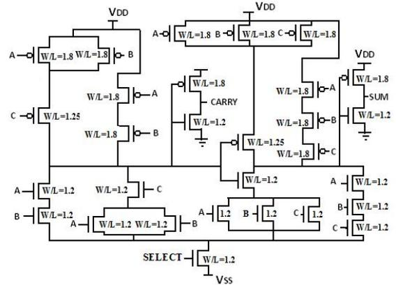
Figure 5. Proposed 1 bit full adder (Design2) circuit with sleep transistor
