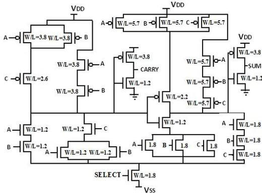
Figure 2. Proposed full adder (Design1) circuit with sleep transistor
